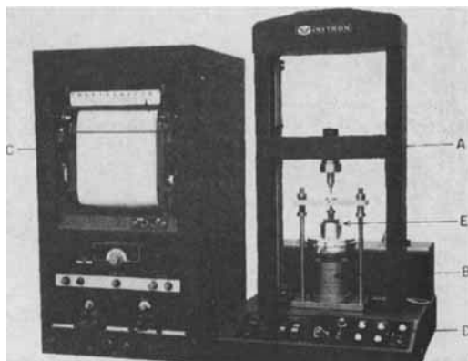
Fig. 1.—Instron universal testing instrument equipped with compression fixture. Key: A, crosshead; B, load cell; C, recorder; D, control panel; E, fixture.
